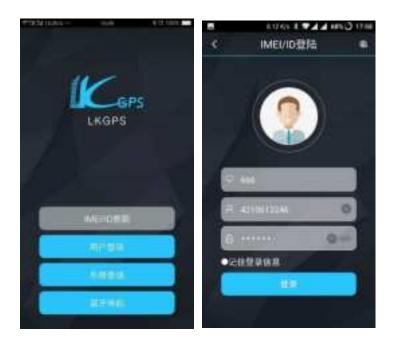
Select "IMEI/ID login" for the first time, select "666" for the address bar in the first column, and input the 10-digit number on the barcode of the device. The default password is 123456.
