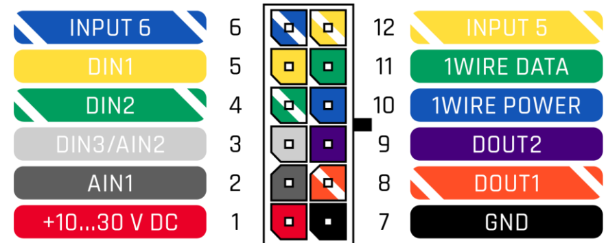
Figure 2 FMB120 2x6 socket pinout
