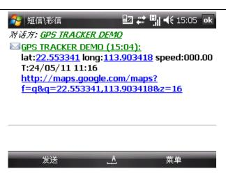
\*Tracking location, When GPS signals is weak, the position of latitude and longitude included in the SMS is the position that the tracker received GPS signals at last. If it is different with its exact current location, pay attention to check the time included in the SMS you got.
