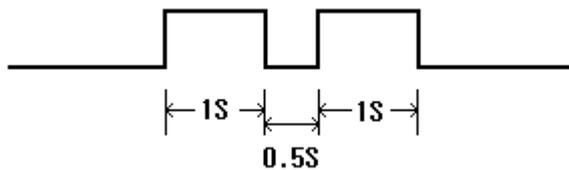
Time for activation and deactivation is configurable by PULSE\_ON and PULSE\_OFF in Service Parameter.
