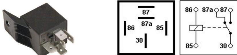
10 Figure Relay pinout
