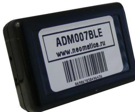
Figure 1 - View of the tracker (the wires are not shown)
