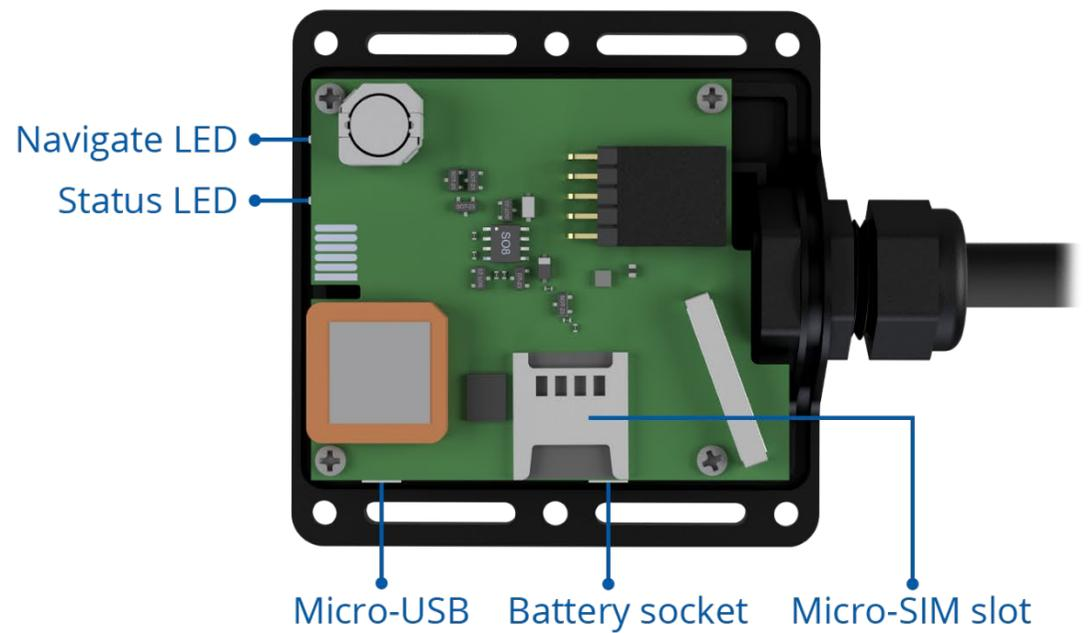
Figure 1 FMB204 device view
