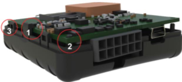
Once the PCB is attached to the pins, place the top of the housing on one side of the device as shown in the image below. Then simply push the other side down until you hear a clicking sound and the housing is closed.
