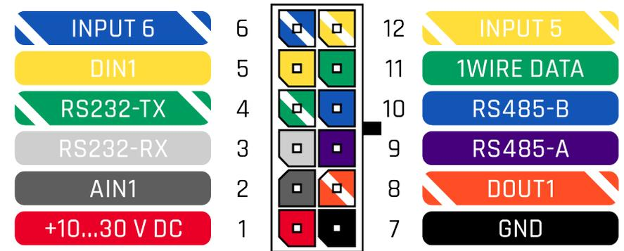
**Figure 2 FMB125 2x6 socket pinout**
