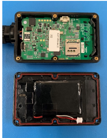
Figure 2: Remove the ST4340LC lid
