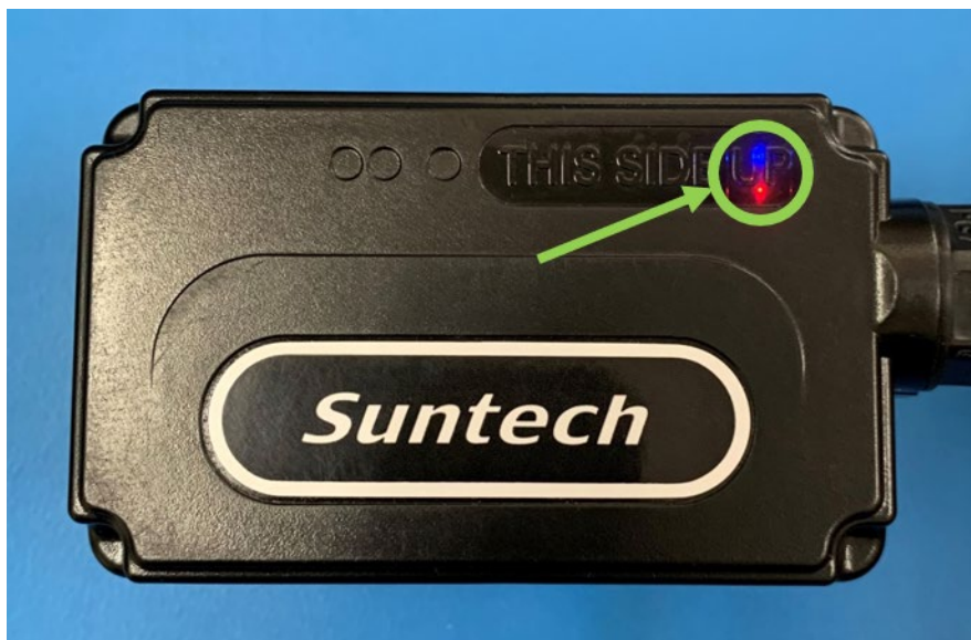
Figure 6: Red and blue LEDs will blink when power is applied
