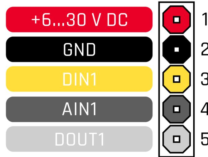
**Figure 2 FMB920 pinout**
