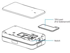
1. Find the notch and remove the upper cover and TPU part.
