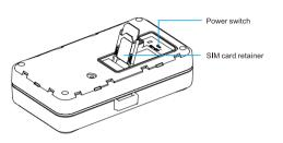
2. Slide the retainer backward and rotate it up, and insert SIM card into it, then rotate it down and slide it frontward.
