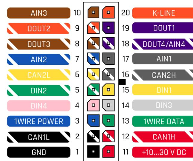
Figure 2 FMC640 pinout
