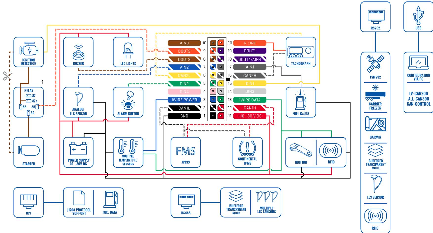
Figure 3 FMC640 Wiring scheme
