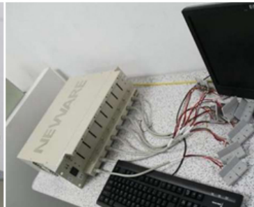
Battery life testing machine
