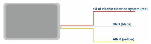
Figure 2 - Color marking of the tracker wires
