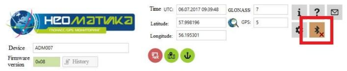
Figure 6 – ADM Configurator: the "disable device" button
