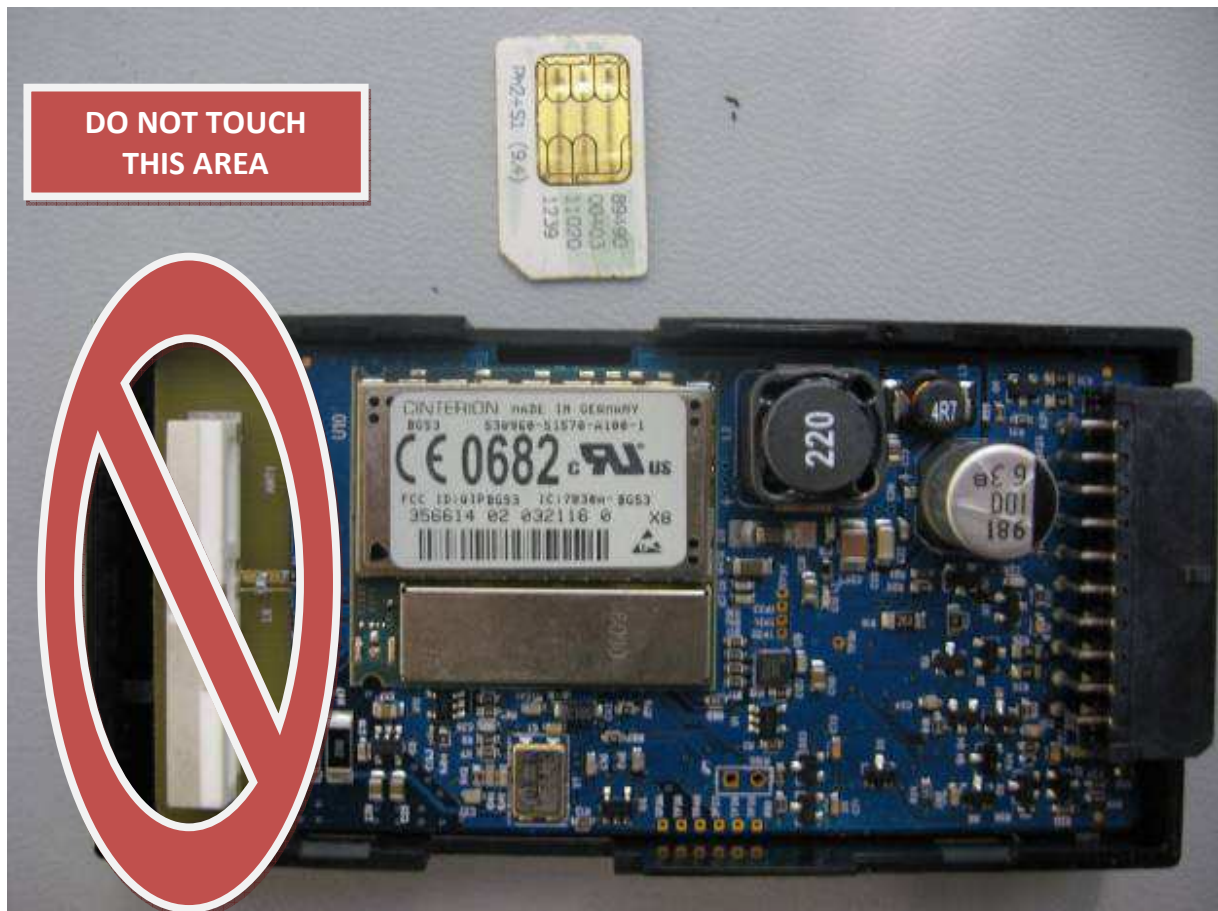
Figure 12 - LMU-2x30™ SIM Alignment
