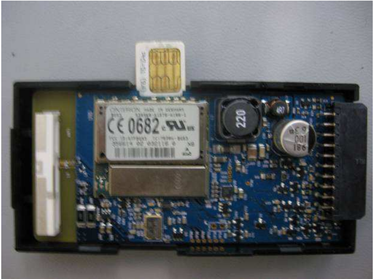
Figure 13 - LMU-2x30™ - Partially Inserted SIM
