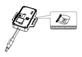
4. Close the SIM card cover and connect the device with the external power line which will be used to charge the terminal and built-in battery.
