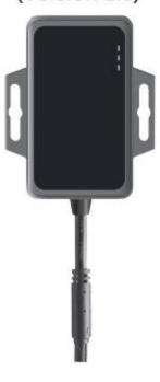
One side of the device is marked "THIS SIDE TOWARDS SKY", place the unit upside down will result in connection issues.
