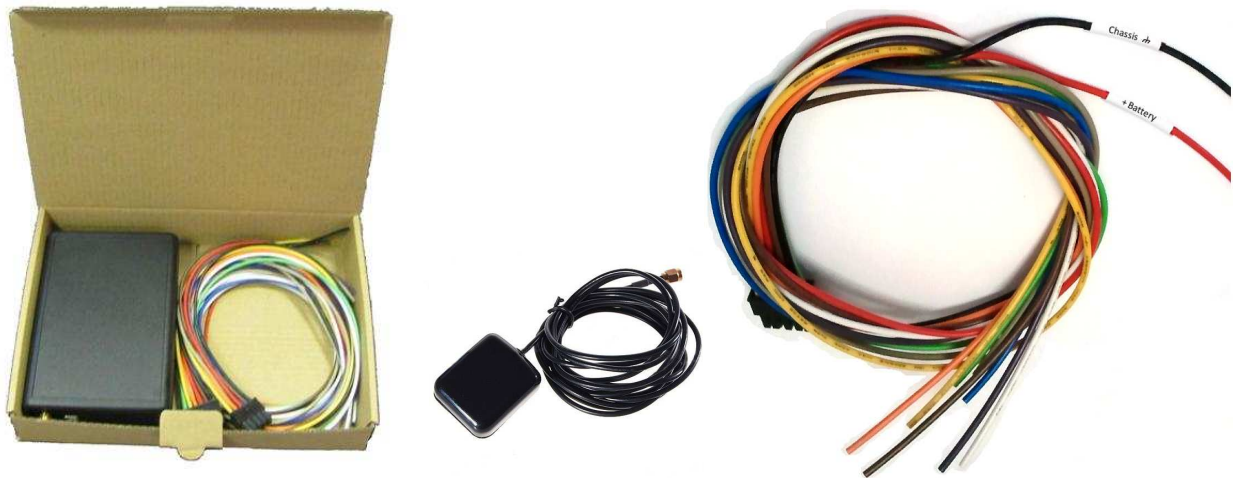
Figure2. FM-Pro3 device, Power, I/O cables and GPS antenna.
