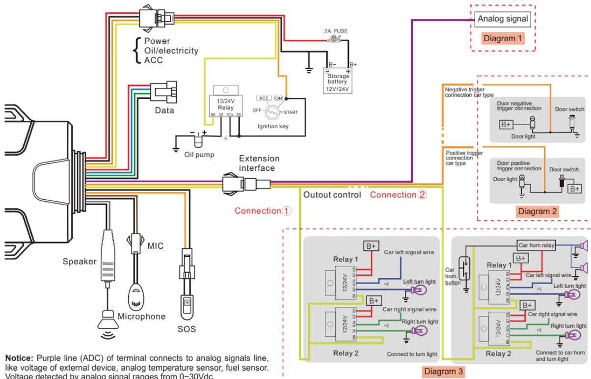
**Notice:** Purple line (ADC) of terminal connects to analog signals line, like voltage of external device, analog temperature sensor, fuel sensor. Voltage detected by analog signal ranges from 0~30Vdc.
