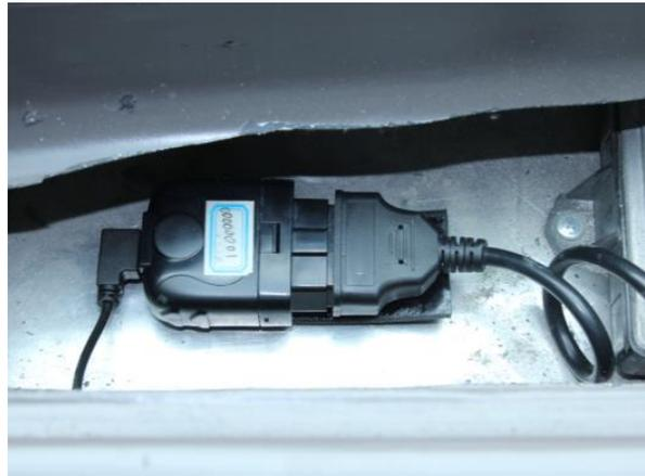
For vehicles do not have an OBD port, please use power cable to connect vehicle battery and configure the device with tracker mode.
