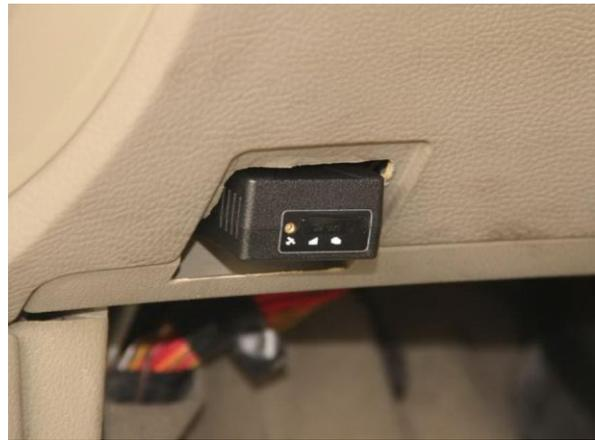
If the OBD port cover can not be closed back after device plugged in, please use OBD extension cable and mount the device in proper place.
