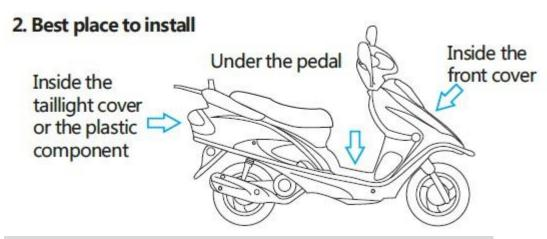
NOTE: The GPS signal will be attenuated if the device is installed under the driver seat.
