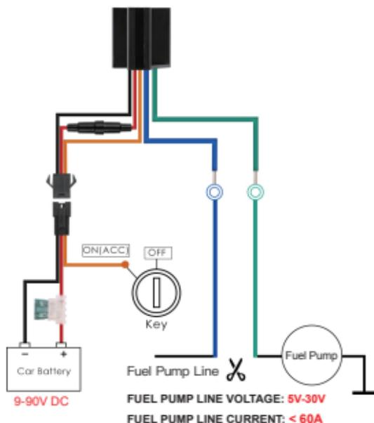
**NOTE** ⚠️⚠️⚠️ : After installed SIM card correctly , it is very important to connect the tracker with external power no less than 12V for power supply before operation!
