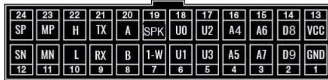
Fig. 3 – Main connector pinout
