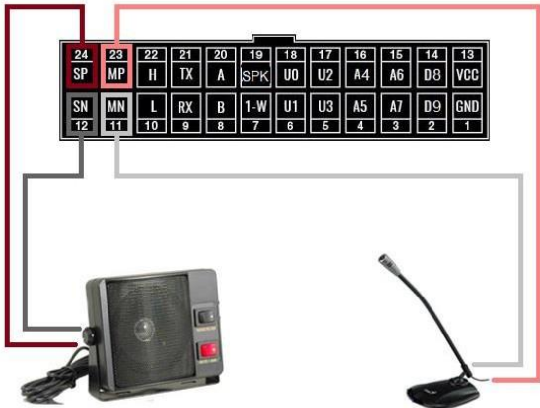
Figure 9 – Diagram of connecting the microphone and speaker
