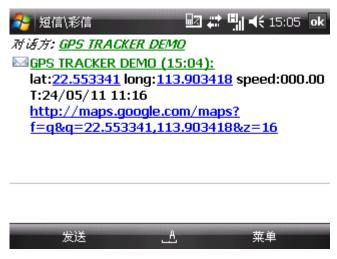
\* Tracking location, when no GPS signal, the SMS includes the last valid latitude & longitude as well as the LAC code of current position, the LAC code can be input in the column of "manual track" menu of web platform to check the location.
