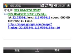
\*When lost fix to satellites, the message will includes the last known GPS position and the LAC code of current position as well.
