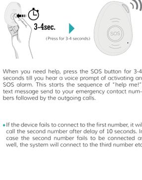
Between each call, it will have 10 seconds delay, during this time, user can stop call sequence or prevent a possible false alarm by pressing the SOS button. The receiver of the call can also stop call sequence by pressing 1 on their mobile phone during two-way talking.
